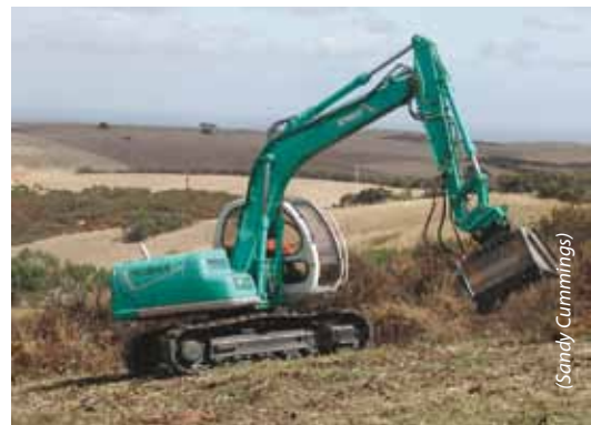
Groomer head on an excavator, Delamere, South Australia
